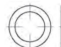
Rondelle plane Gaz Cuivre recuit Annealed Copper flat Plate Rondella in Rame
